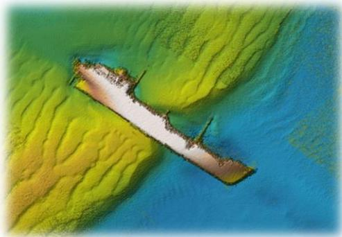
*A wreck detected by side scan sonar*
